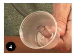
Slide the end of the rubber tubing (not attached to the funnel) into the hole in the portion cup.
