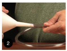
Attach a length of rubber tubing to the narrow end of the funnel by squeezing the funnel into the tubing.
