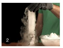
Make sure that you have pieces of dry ice that are small enough to fit inside your graduated cylinder. Once you've created the small pieces, drop a few into the graduated cylinder.
