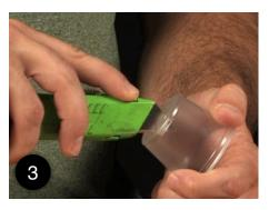
Use the utility blade to cut a hole in the bottom of a small plastic portion cup just large enough to fit the rubber tubing.
